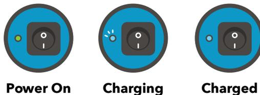
2. The green light on the front of the Power Pack indicates the power is on. The blinking blue cradle lights indicate the robots are charging.
